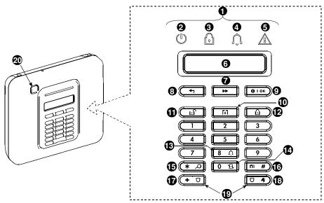
Figure 1a. PowerMaster-10 G2 Controls and Indicators
