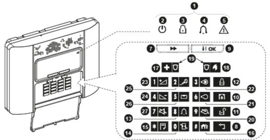
Figure 1b. PowerMaster-30 G2 Controls and Indicators
