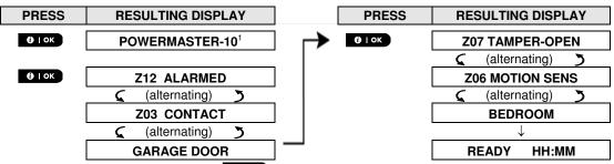
In response to additional clicking of the button, the display shows details of other events retained in open tamper (if any), or reverts to its initial state (see A above).
